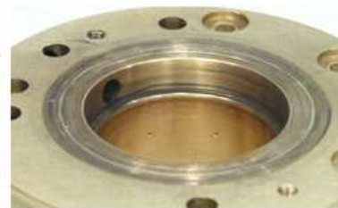
Thrust Bearing Rub
